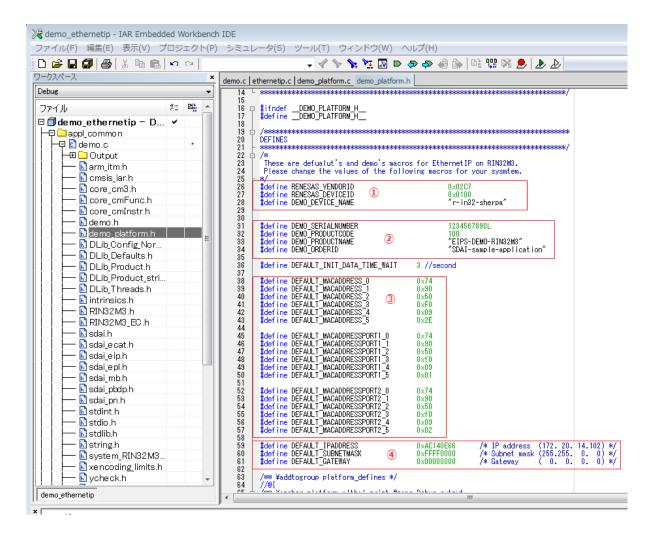
There are four sections of this file that must be modified to customize an application. The explanation below elaborate further on the changes required for "demo\_platform.h" header file.
