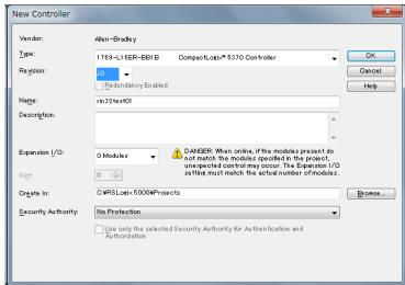
In order to add the r-in32 EtherNet/IP sample application to the IO scan list right-click new module on the Ethernet icon under the I/O configuration folder in the RSLogix 5000 project.
