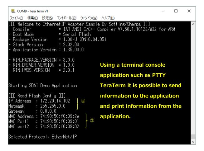
When the Ethernet/IP device stack application runs on the R-IN32M3 evaluation board for the first time the values shown in the above screenshot are written to the flash ROM of R-IN32M3 on the evaluation board, and the application will start with those values.
