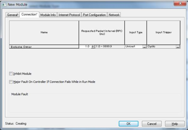
The IO configuration in the EtherNet/IP scanner must correspond to the IO configuration defined in the Sherpa application running on R-IN32M3.
